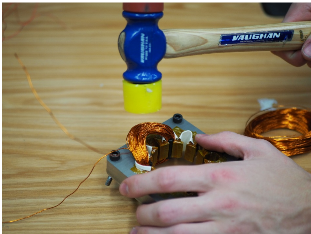
Figure 42. Use a mallet to form the winding.
