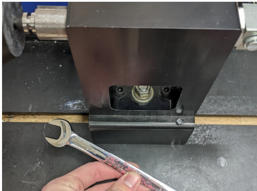
Figure 29. Move the chuck into the jig w/ 9/16" wrench.
