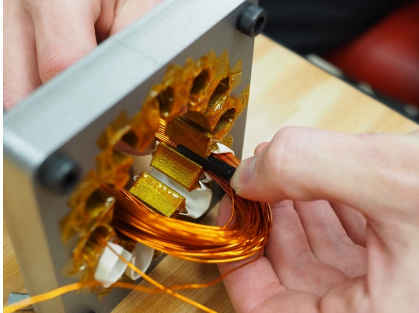
Figure 39. Inserting winding retainer into stator slot.
