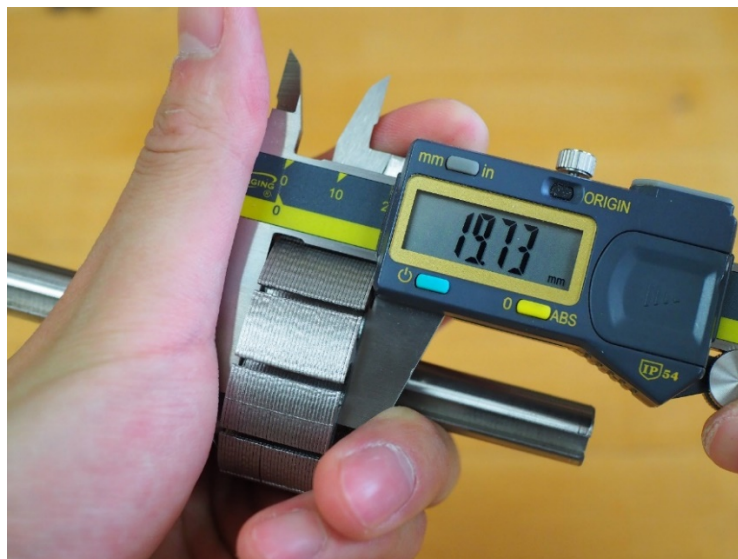
Figure 9. Ensure the rotor lamination thickness is at or no greater than 20 [mm].
