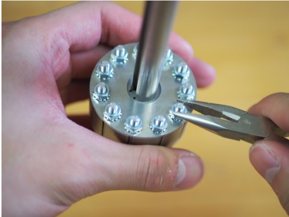
Figures 15 (Left) and 16 (Right). Tightening both sides of the aluminum standoffs.
