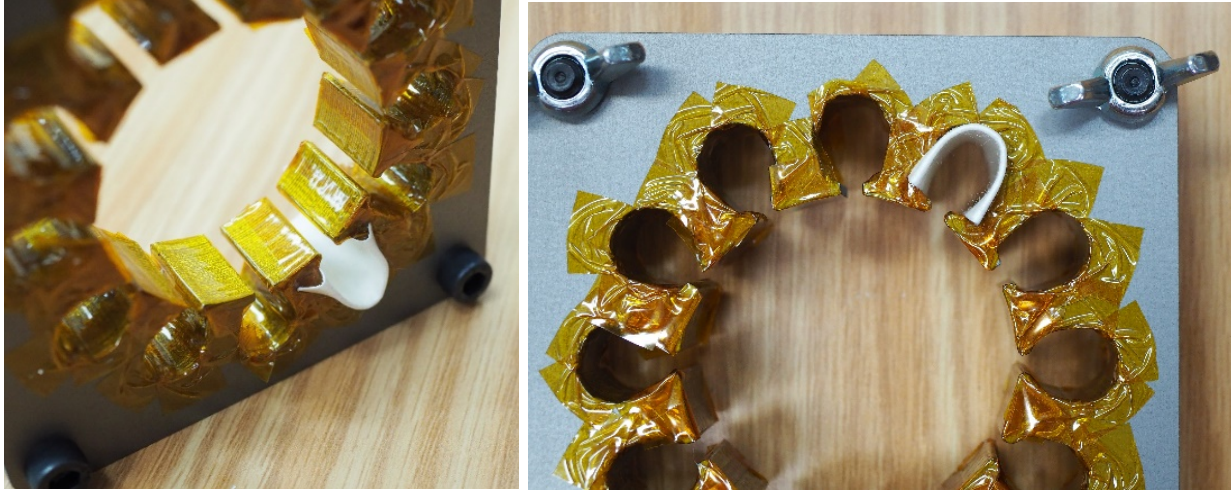
Figure 23 (Left) and Figure 24 (Right). Polyimide tape applied to stator slots
