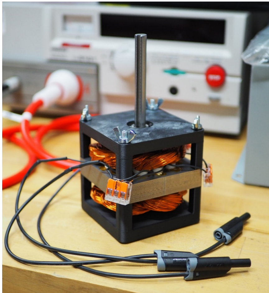
Figure 1. Fully assembled 4-pole, 12 slots, squirrel-cage rotor induction motor.
