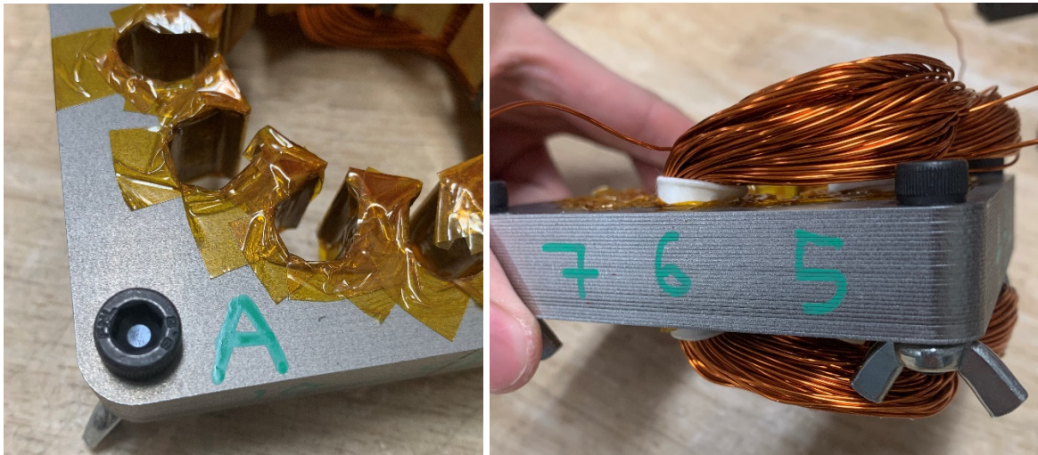
Figure 36 and 37. Labeling side and slot numbers on stator lamination.
