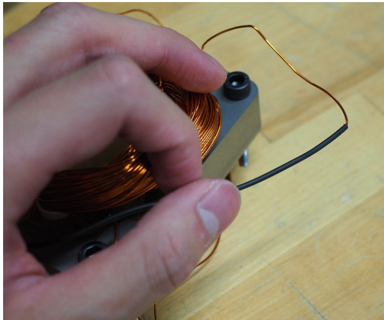
Figure 47. Inserting heat shrink tube to coils.
