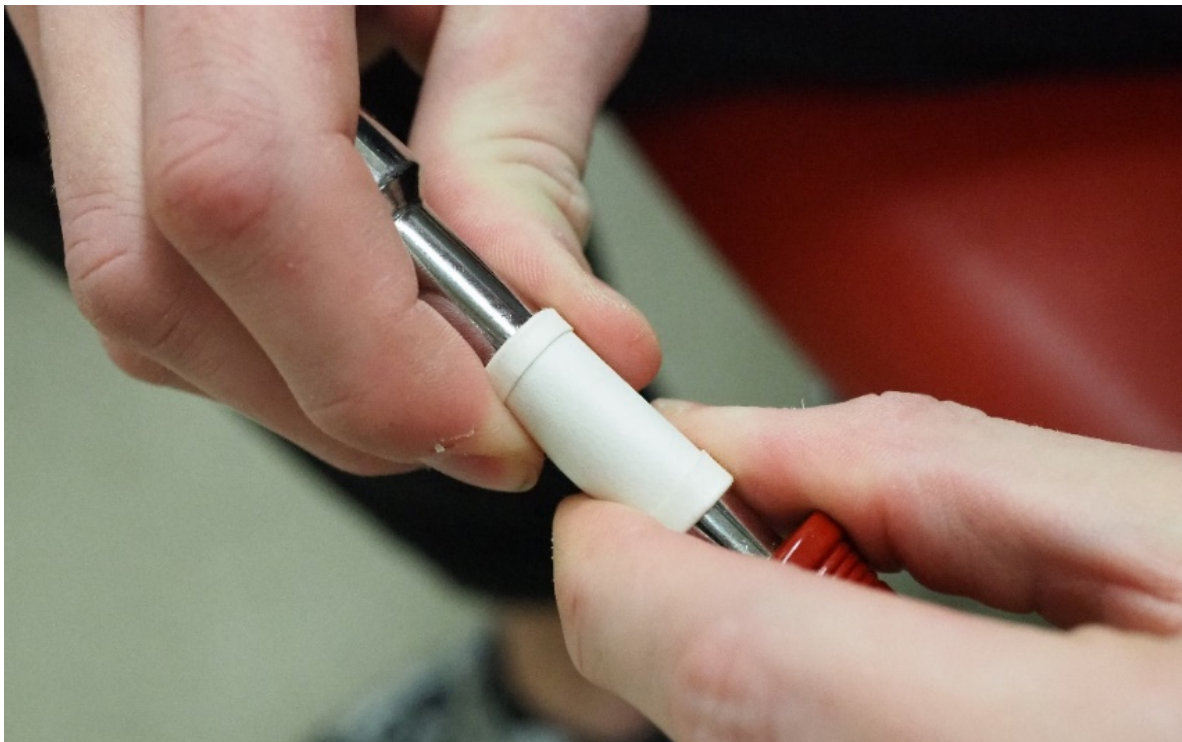
Figure 22. Forming stator insulation paper.
