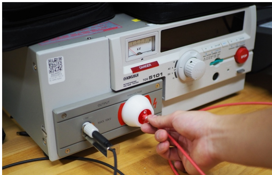
Figure 48. A high-pot test machine.
