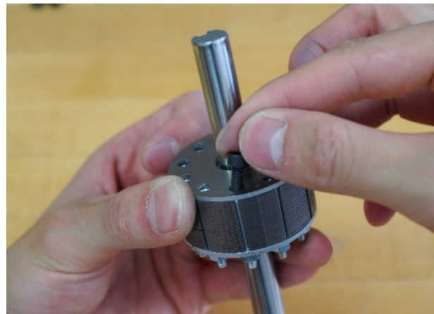
Figures 13 (Left) and 14 (Right). Applying the Loctite and placing the fasteners in the female end of the standoff.
