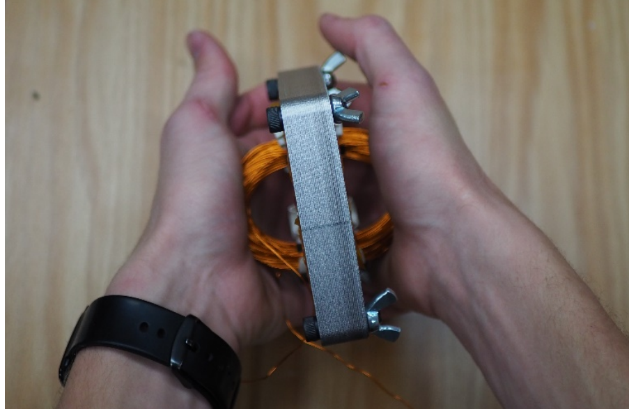
Figure 41. Form the winding shape by hand.
